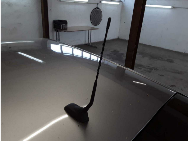
Damage #1: Roof: Stub aerial - Damaged - Replace
