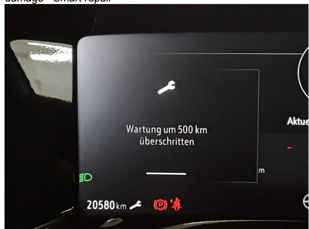
Damage #4: Misc.: Inspection / maintenance - Due - Replace
