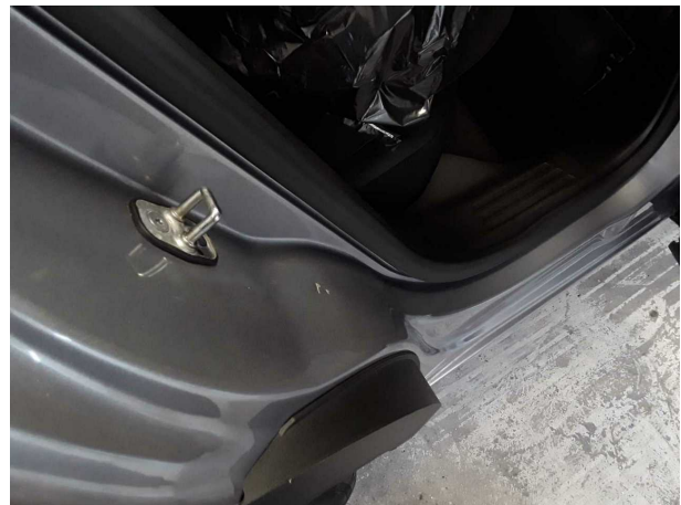
Damage #3: Side panel - rear right side: Sill - Dent / paintcoat damage - Smart repair
