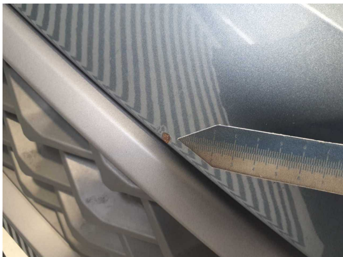
Damage 12: Bonnet: Bonnet - Corrosion - Paint
