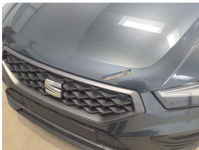
Damage 12: Bonnet: Bonnet - Corrosion - Paint
