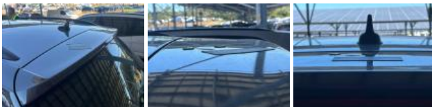
Roof, Hail damage, Repair and paint (complete)
