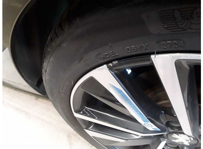
Damage 8: Wheel / tyres: Alloy rim - rear left side - Scratched - Loss in value
