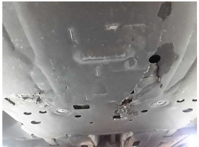
Damage 9: Body: Underbody panelling - Damaged - Replace
