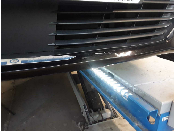
Damage 10: Front bumper: Front bumper - Damaged - Replace
