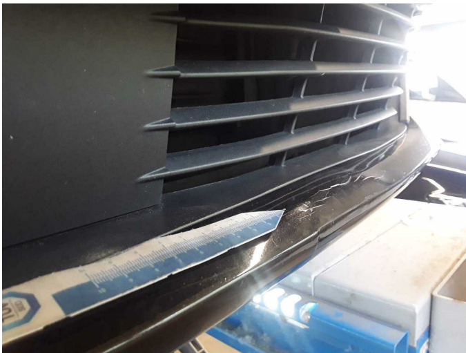
Damage 10: Front bumper: Front bumper - Damaged - Replace
