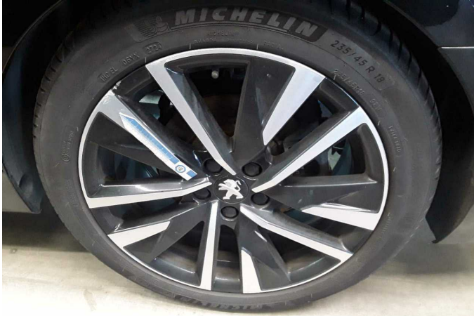
Damage 8: Wheel / tyres: Alloy rim - rear left side - Scratched - Loss in value
