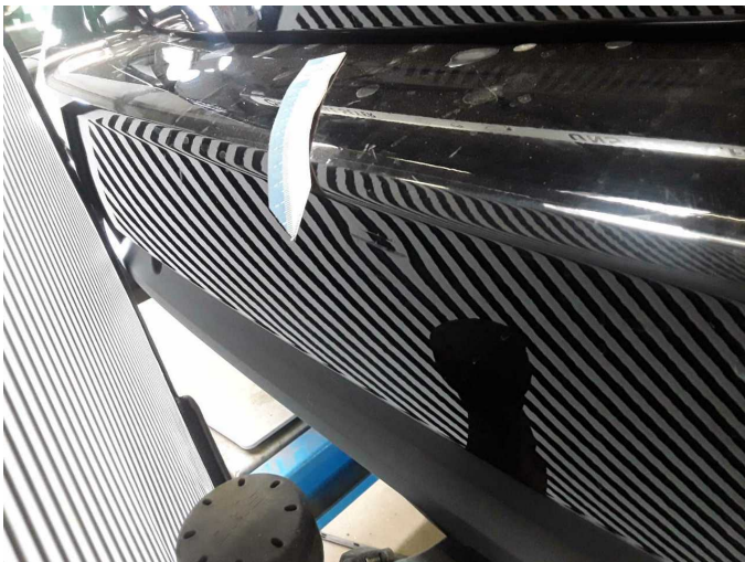
Damage 3: Rear bumper: Rear bumper - Dent / paintcoat damage - Smart repair
