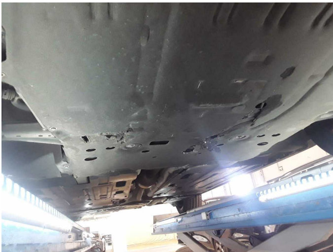
Damage 9: Body: Underbody panelling - Damaged - Replace
