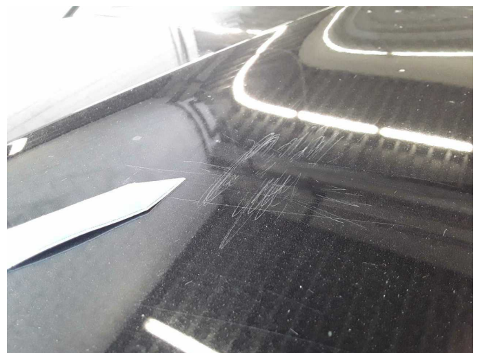
Damage 10: Bonnet: Bonnet - Scratched - Paint
