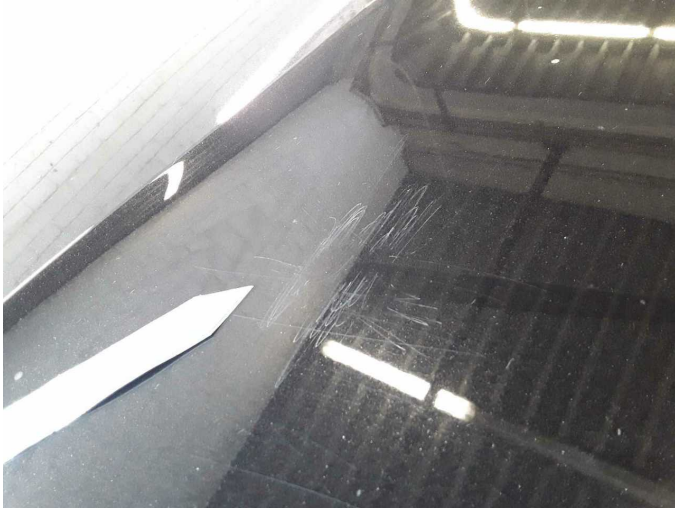
Damage 10: Bonnet: Bonnet - Scratched - Paint
