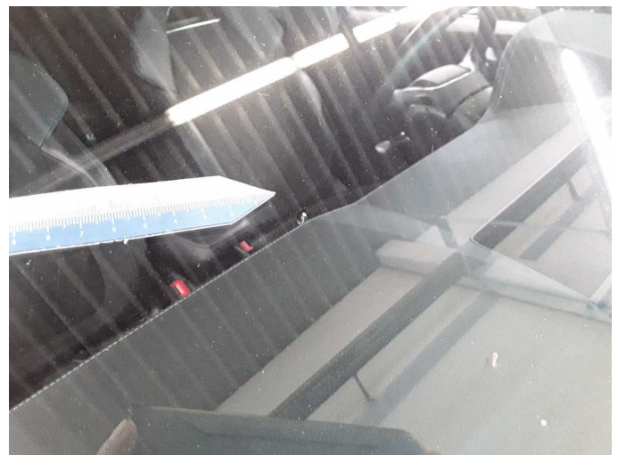
Damage 12: Vehicle glazing: Windscreen (Rissbildung) - Stone chips - repair according to calculation
