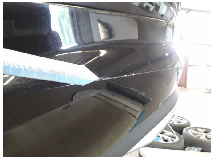
Damage 6: Rear bumper: Rear bumper - Scratch(es) - Paint
