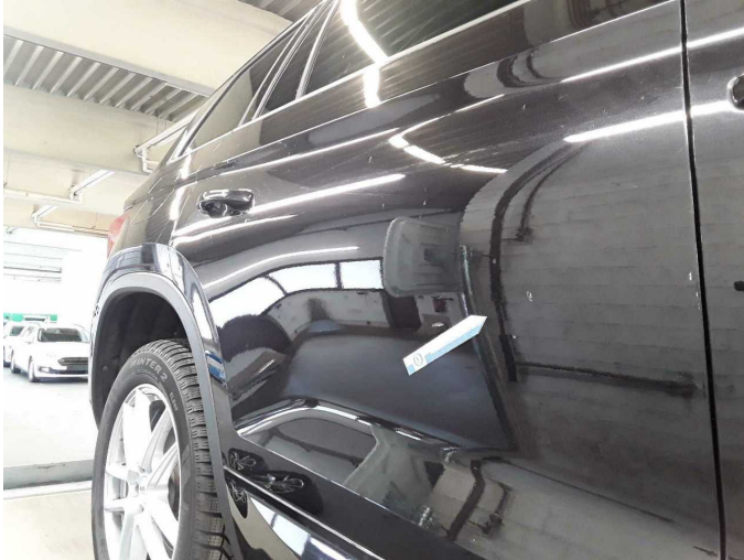
Damage 9: Door - rear right side: Door - Dent / paintcoat damage - Repair and paint
