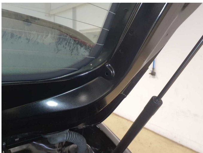
Damage 1: Trim / covers: Trim / covers (Hutablagen Halterung) - Missing - Replace
