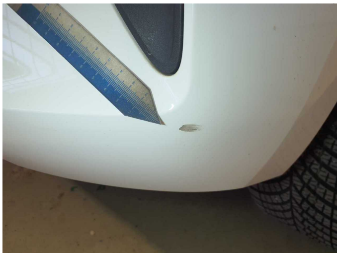
Damage 7: Rear bumper: Rear bumper - Scratch(es) - Paint
