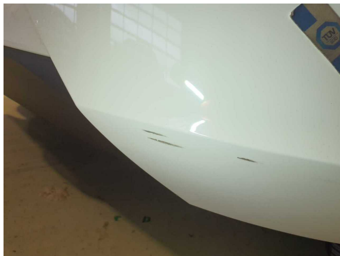
Damage 7: Rear bumper: Rear bumper - Scratch(es) - Paint
