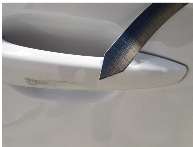
Damage 2: Door - front right side: Door handle - outside - Scratch(es) - Smart repair
