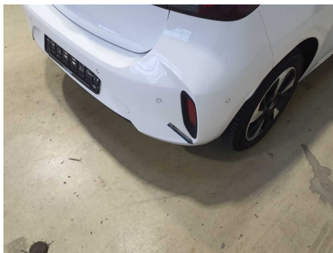
Damage 7: Rear bumper: Rear bumper - Scratch(es) - Paint
