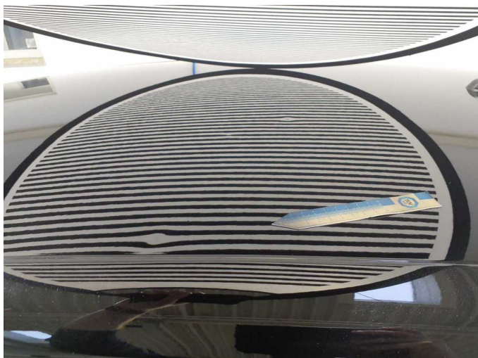
Damage 5: Roof: Roof - Dent / paintcoat damage - Smart repair
