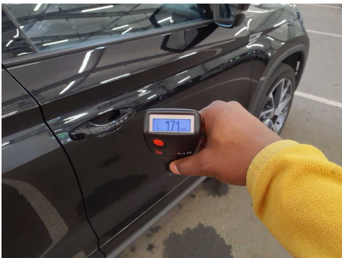
Repainting 1: Door - front right side
