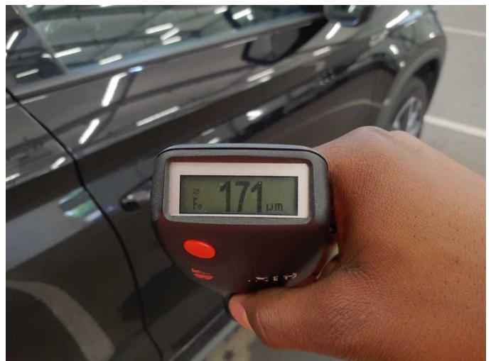
Repainting 1: Door - front right side
