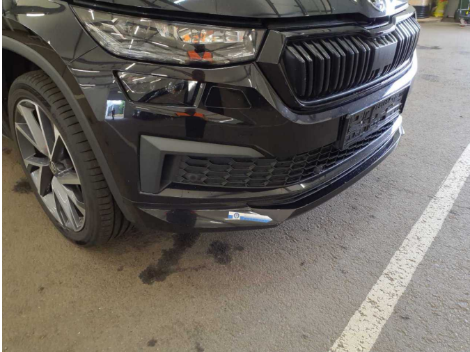
Damage 2: Front bumper: Spoiler - Scratched - Replace
