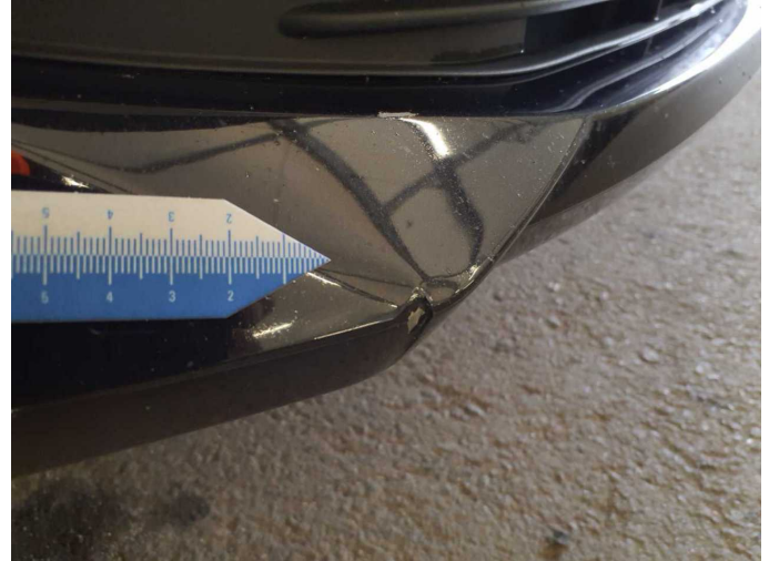
Damage 2: Front bumper: Spoiler - Scratched - Replace
