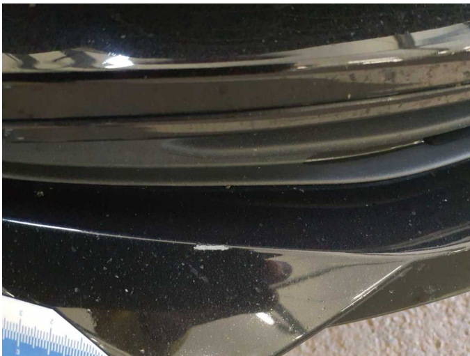
Damage 2: Front bumper: Spoiler - Scratched - Replace
