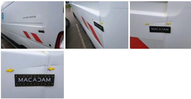
Car body corner RL, Dent(s) and scratch(es), Repair and paint (complete)
