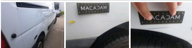
Side panel moulding R, Missing, Replace
