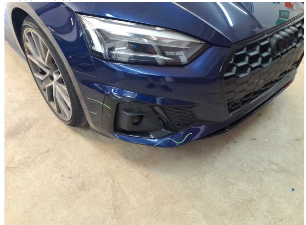
Damage #8: Front bumper: Front bumper - Scratched - Loss in value
