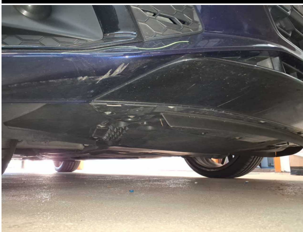
Damage #8: Front bumper: Front bumper - Scratched - Loss in value
