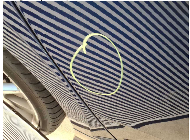
Damage #14: Door - rear right side: Door - Dent / paintcoat damage - Repair and paint
