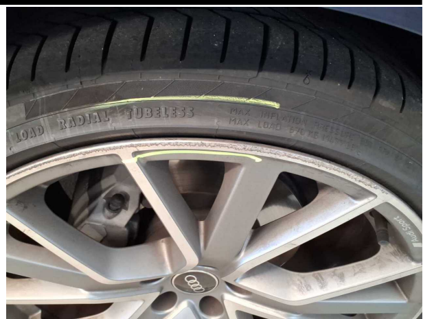
Damage #9: Wheel / tyres: Alloy rim - front right side - Scratched - Loss in value
