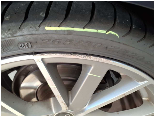
Damage #10: Wheel / tyres: Alloy rim - rear right side - Scratched - Loss in value
