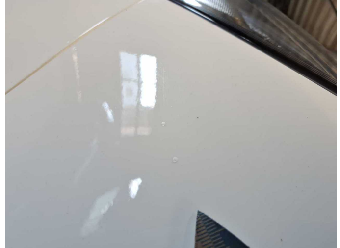
Damage 7: Mudguard - left side: Mudguard - left side - Stone chips - Repair and paint
