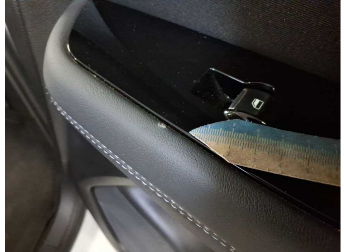
Damage 5: Trim / covers: Door trim - front right side - Broken / torn - Smart repair
