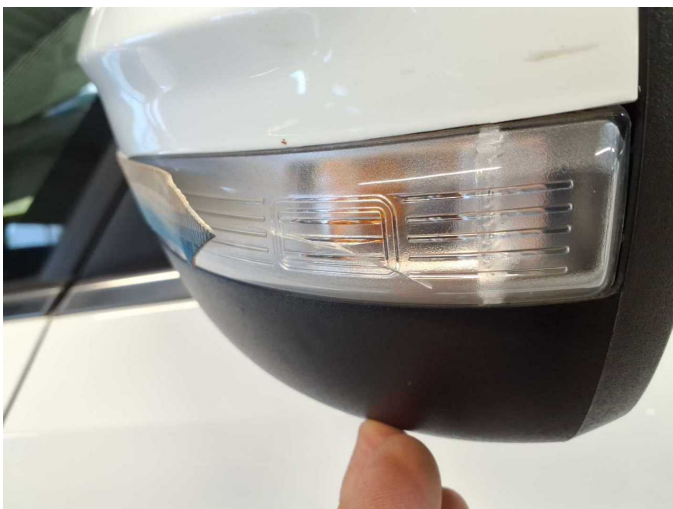
Damage 2: Indicator - front: Mirror - left side - Broken / torn - Replace
