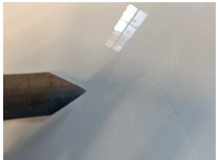
Damage 6: Mudguard - right side: Mudguard - right side - Stone chips - Repair and paint
