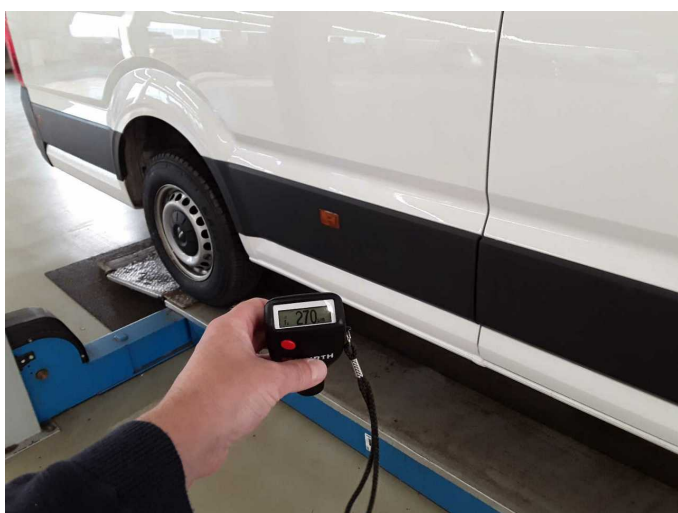
Side panel - rear right side: 270 µm
