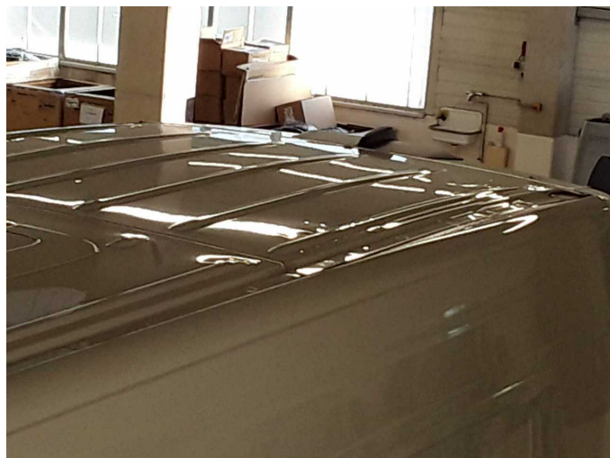
Damage 5: Roof: Roof - dent(s) - Repair and paint
