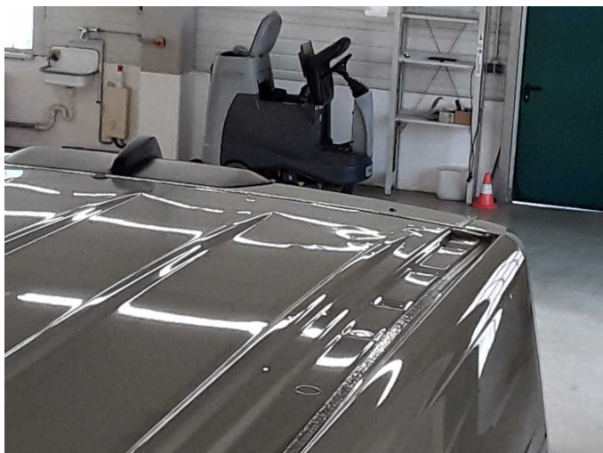
Damage 5: Roof: Roof - dent(s) - Repair and paint
