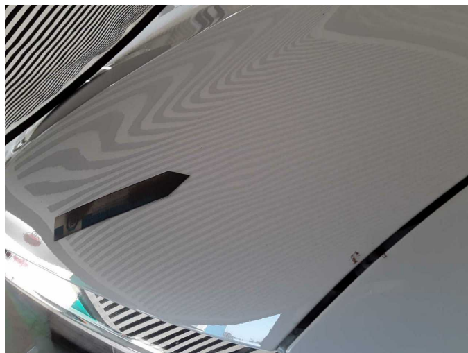
Damage 1: Bonnet: Bonnet - dent(s) - Smart repair
