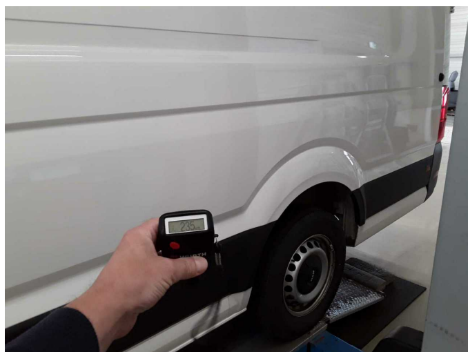
Side panel - rear left side: 235 µm
