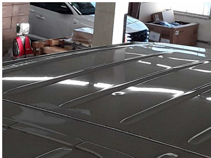
Damage 5: Roof: Roof - dent(s) - Repair and paint
