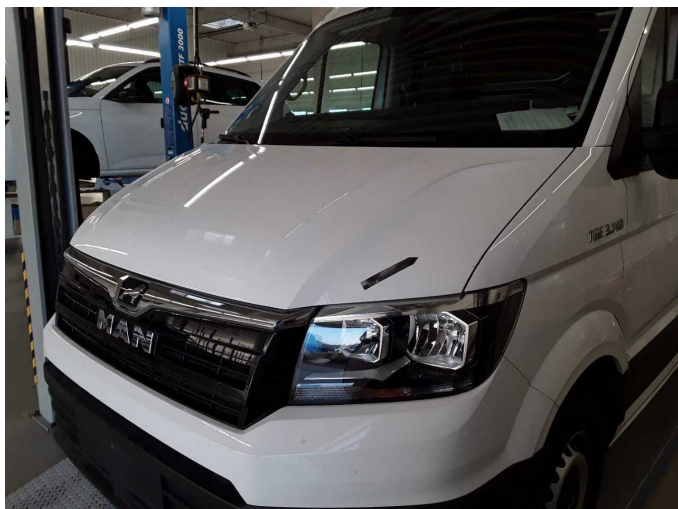
Damage 1: Bonnet: Bonnet - dent(s) - Smart repair
