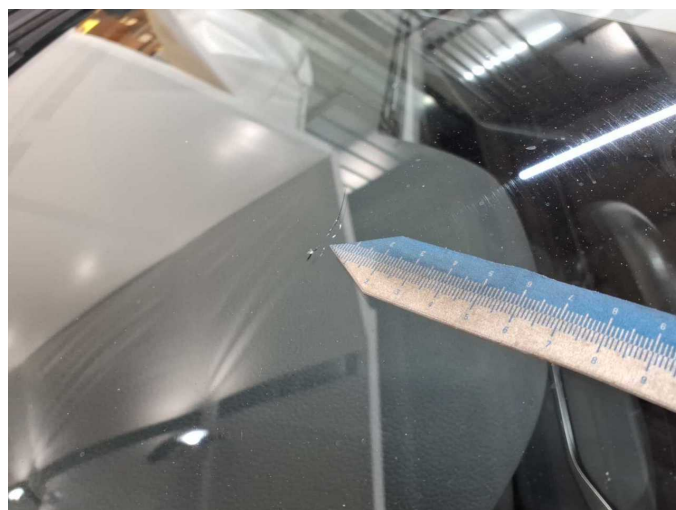
Damage 8: Vehicle glazing: Windscreen - Stone chips - Replace
