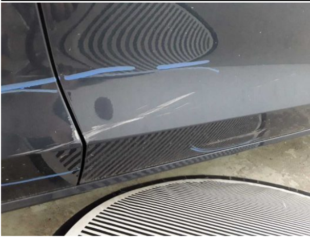
Damage #19: Door - front right side: Door - Deformed - Replace
