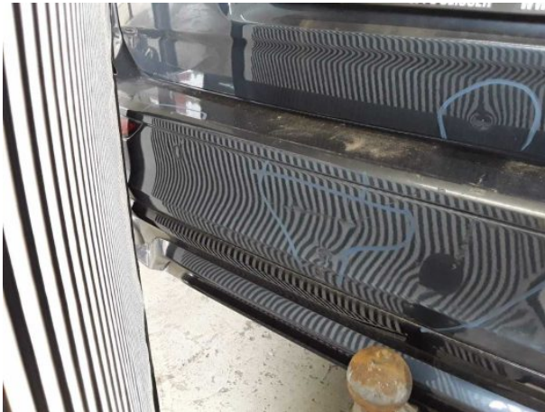
Damage #17: Rear bumper: Rear bumper - Deformed - Replace
