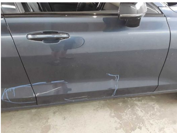
Damage #19: Door - front right side: Door - Deformed - Replace
