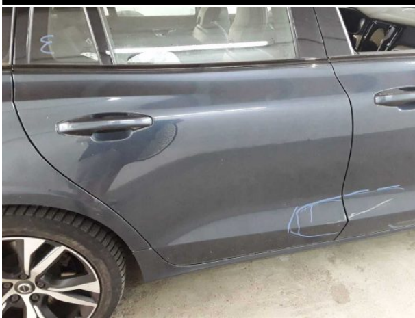
Damage #14: Door - rear right side: Door - Scratched - Repair and paint
