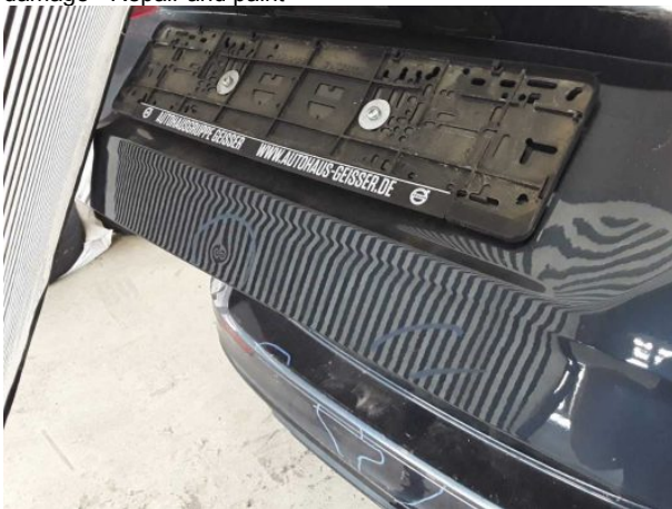
Damage #16: Boot lid / rear door: Boot lid - Dent / paintcoat damage - Repair and paint
