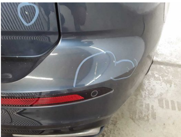
Damage #17: Rear bumper: Rear bumper - Deformed - Replace
