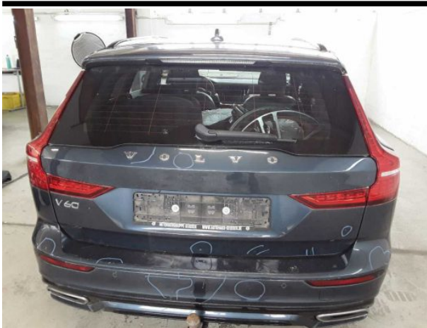
Damage #16: Boot lid / rear door: Boot lid - Dent / paintcoat damage - Repair and paint
