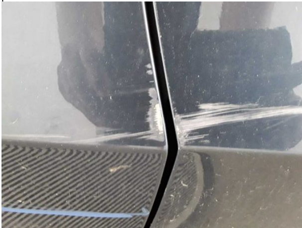
Damage #14: Door - rear right side: Door - Scratched - Repair and paint
