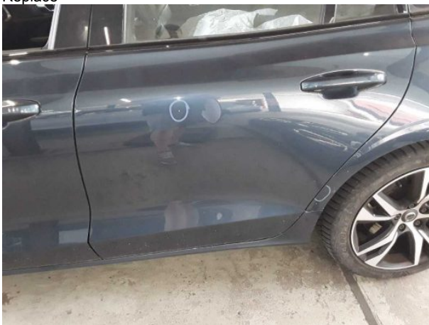
Damage #13: Door - rear left side: Door - Dent / paintcoat damage... Repair and paint
