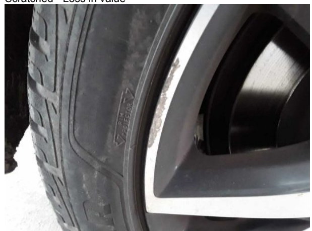
Damage #7: Wheel / tyres: Alloy rim - rear right side - Scratched - Loss in value
