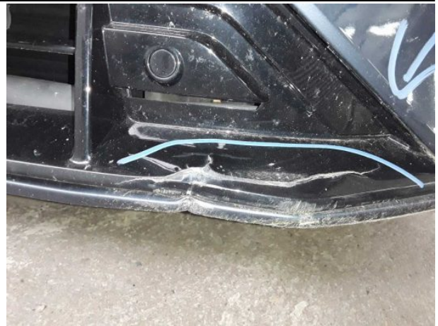
Damage #11: Front bumper: Air-inlet grille (Mitte) - Deformed - Replace
