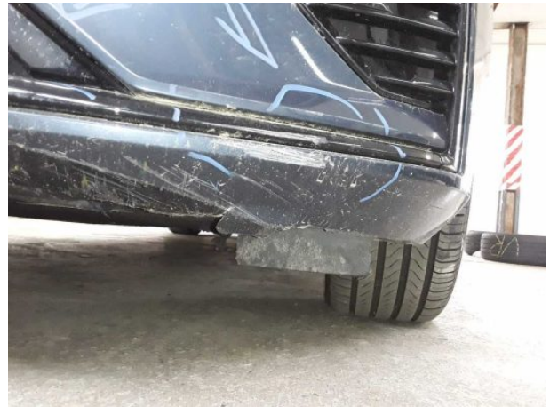
Damage #18: Front bumper: Front bumper - Deformed - Replace
