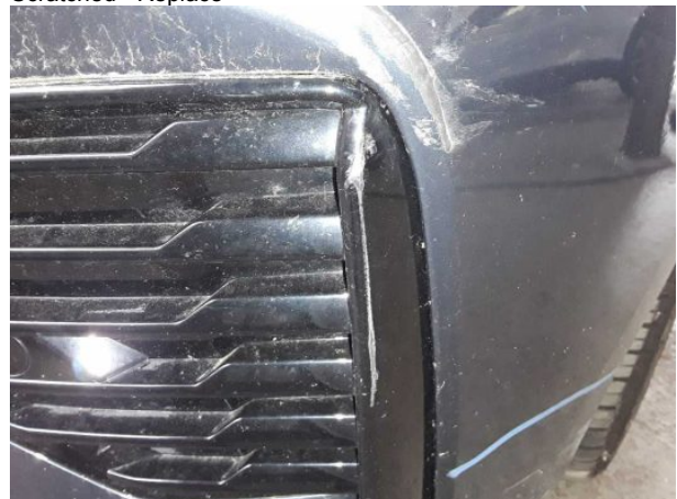
Damage #3: Front bumper: Air-inlet grille (Vorne links) - Scratched - Replace
