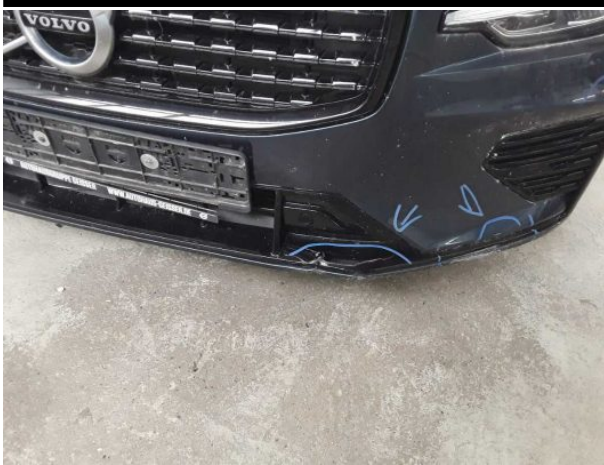
Damage #11: Front bumper: Air-inlet grille (Mitte) - Deformed - Replace
