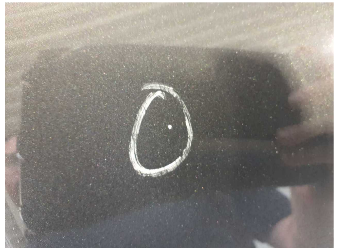
Damage 12: Bonnet: Bonnet - Stone chips - Paint
