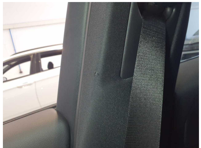
Damage 2: Trim / covers: B-pillar - trim - interior, right side - Scratch(es) - Smart repair
