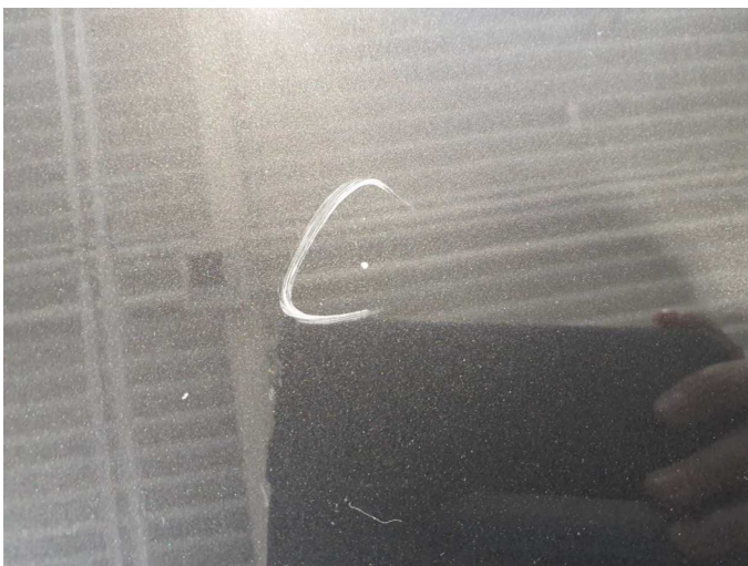
Damage 12: Bonnet: Bonnet - Stone chips - Paint
