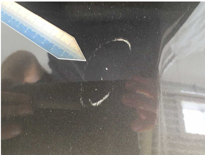
Damage 12: Bonnet: Bonnet - Stone chips - Paint
