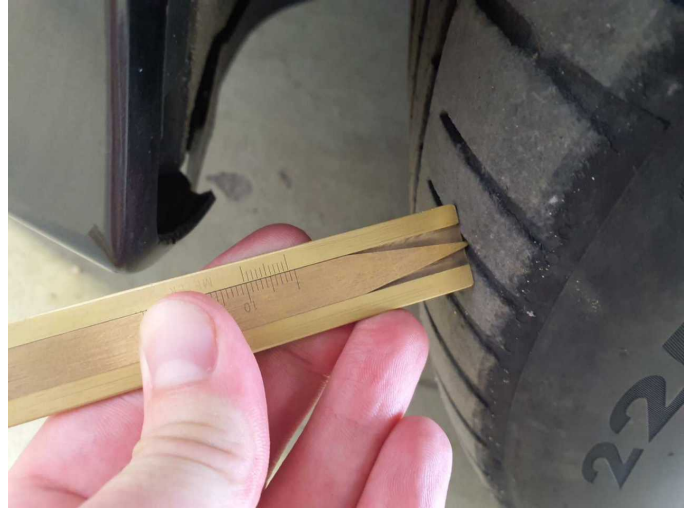
Damage 9: Wheel / tyres: Tyre - front - Worn - Replace
