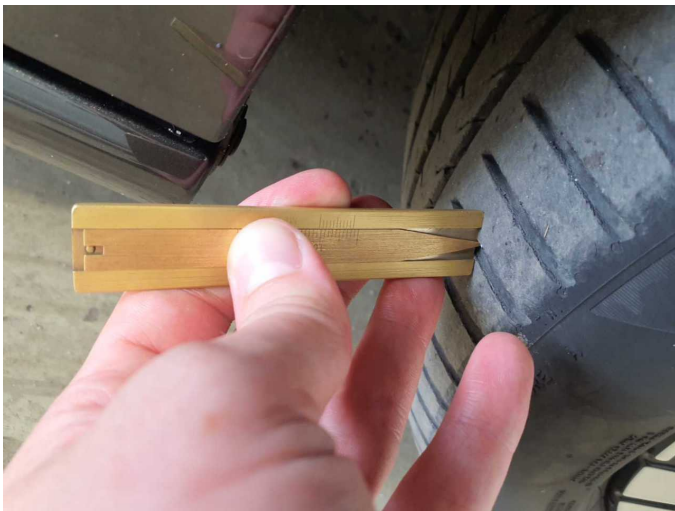
Damage 9: Wheel / tyres: Tyre - front - Worn - Replace
