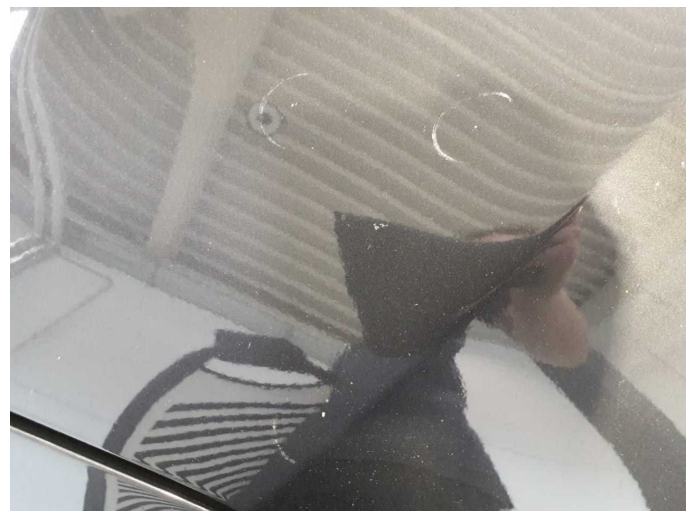
Damage 12: Bonnet: Bonnet - Stone chips - Paint
