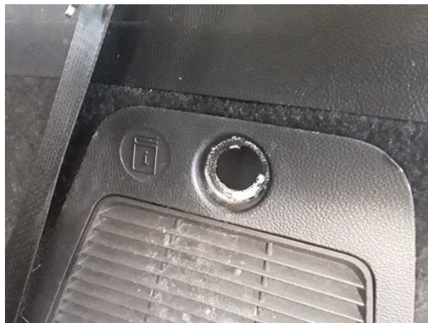
Damage #2: Trim / covers: Boot lining (Deckel rechts) - Damaged - Replace
