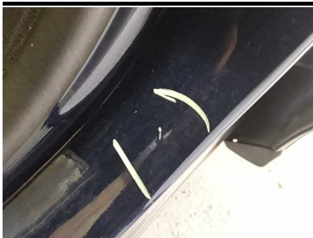
Damage #5: Sill - left side: Sill - Scratched - Smart repair
