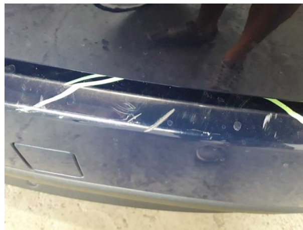
Damage #10: Rear bumper: Rear bumper - Scratched - Paint
