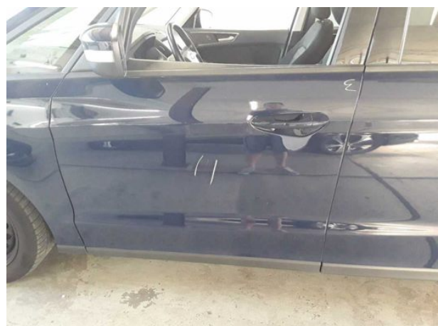
Damage #14: Door - front left side: Door - Scratched - Paint
