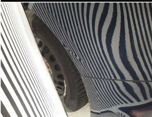
Damage #16: Side panel - rear left side: Side panel - Dent / paintcoat damage - Repair and paint
