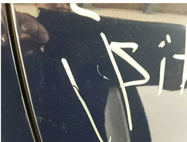
Damage #13: Door - front right side: Door - Scratched - Paint
