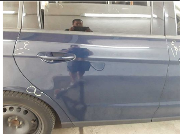
Damage #12: Door - rear right side: Door - Scratched - Paint
