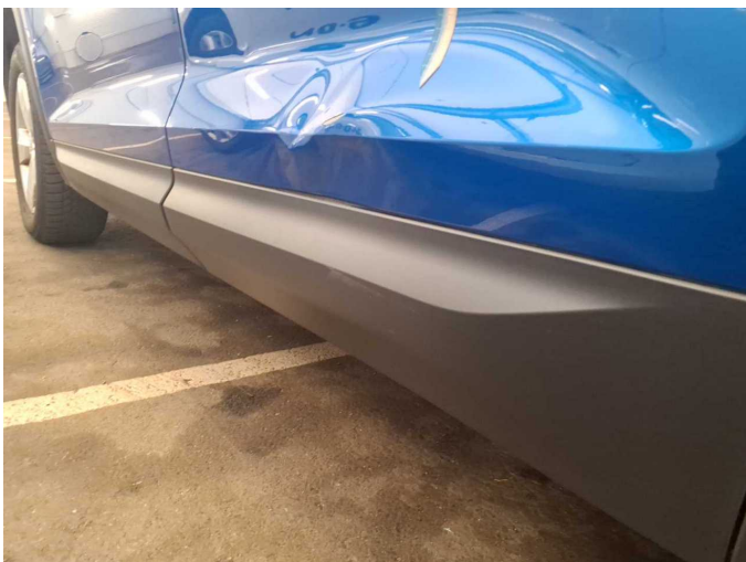
Damage 3: Door - rear left side: Door - Deformed - Replace
