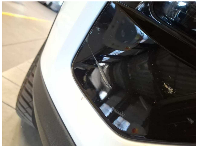
Damage 1: Fog lamp: Fog lamp - front right side (Rahmen) - Scratch(es) - Replace
