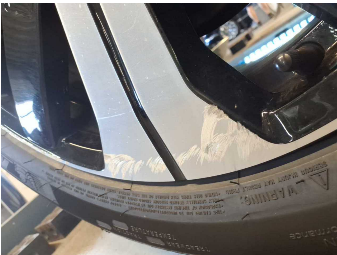
Damage 4: Wheel / tyres: Alloy rim - front left side (Materialabtrag) - Scratched - Replace
