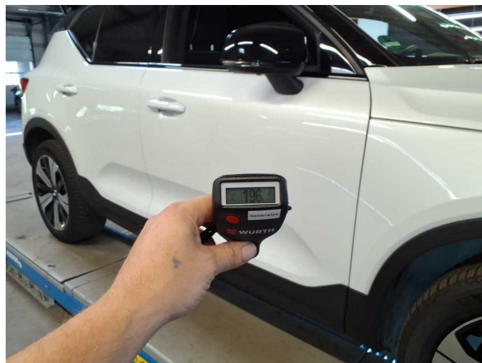
Repainting 4: Door - front right side
