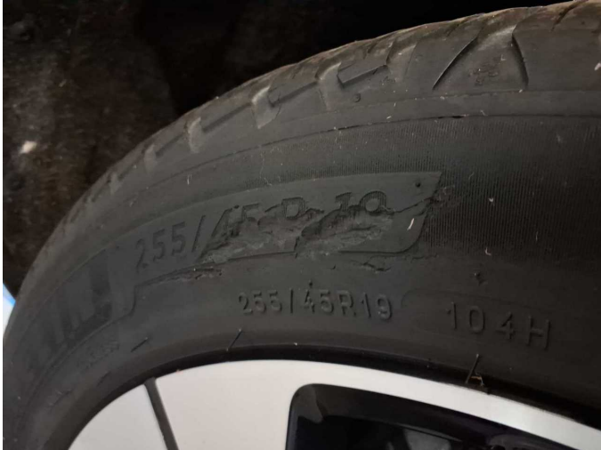
Damage 2: Wheel / tyres: Tyre - rear right side (Flanke) - Damaged - Replace
