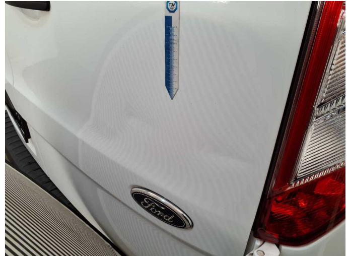
Damage 5: Boot lid / rear door: Rear door - right side - Deformed - Repair and paint
