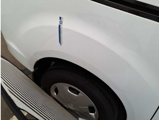
Damage 6: Side panel - rear right side: Side panel (& Lackschaden) - Deformed - Repair and paint
