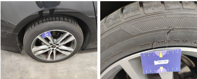
Tyre Rear Right // Replace-cracked
