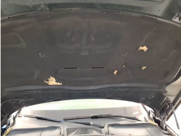
Damage #4: Bonnet: Insulation lining - Damage caused by marte... rodent - Replace
