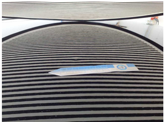
Damage 7: Roof: Roof - dent(s) - Smooth repair work
