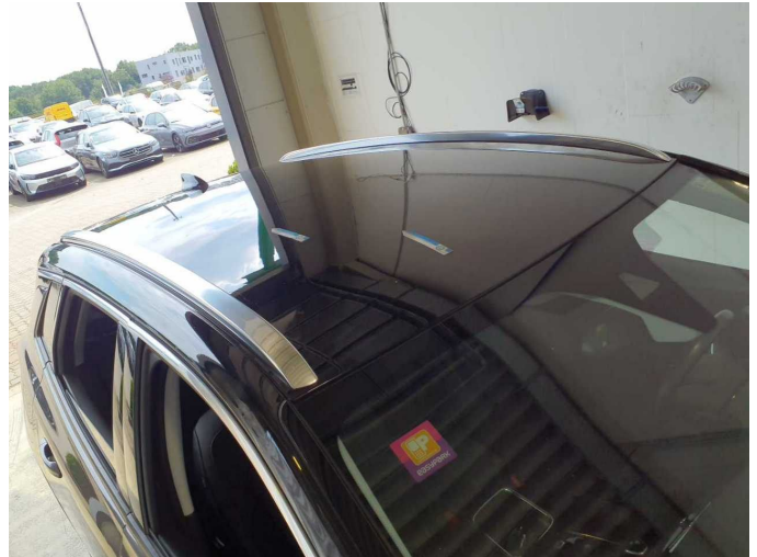
Damage 7: Roof: Roof - dent(s) - Smooth repair work
