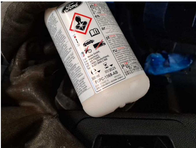
Damage 1: Equipment: Tirefit filler - Expired - Replace
