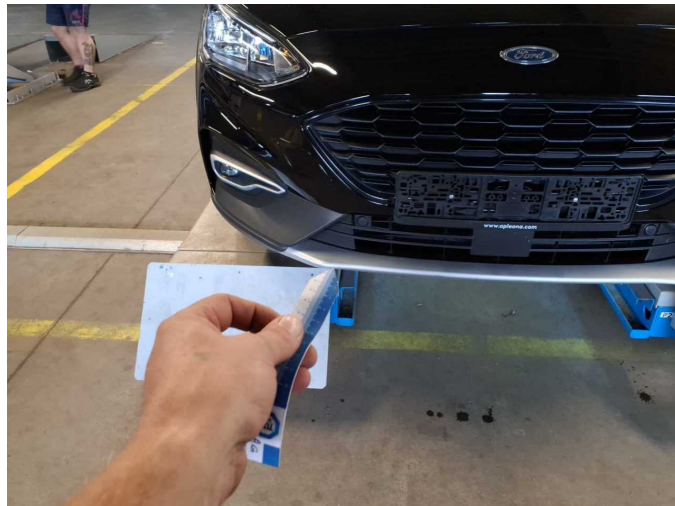
Damage 5: Front bumper: Spoiler - Deformed - Replace
