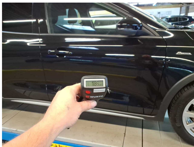
Repainting 3: Door - front right side
