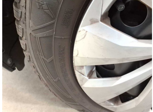
Damage #1: Wheel / tyres: Wheel cover - front left side - Scratch(es) - Replace
