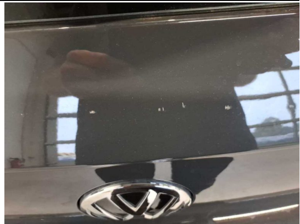
Damage #8: Boot lid / rear door: Boot lid - Scratch(es) - Repair and paint
