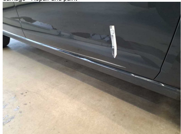
Damage #9: Door - front right side: Door - Dent / paintcoat damage - Repair and paint
