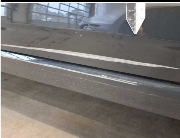
Damage #9: Door - front right side: Door - Dent / paintcoat damage - Repair and paint
