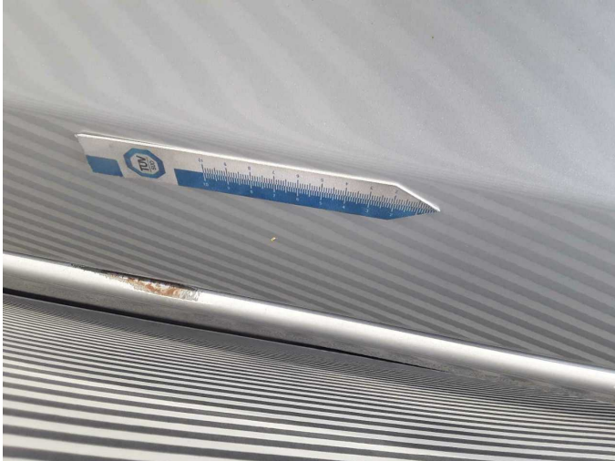
Damage 7: Door - front left side: Door - Dent / paintcoat damage - Smart repair
