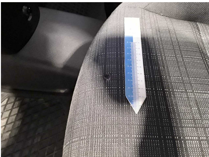
Damage 6: Seat - front: Seat cover - left side - Burn hole (cigarettes) - Smart repair
