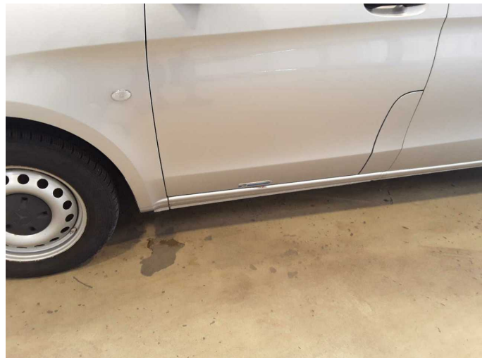
Damage 16: Sill - left side: Sill - Corrosion - Repair and paint
