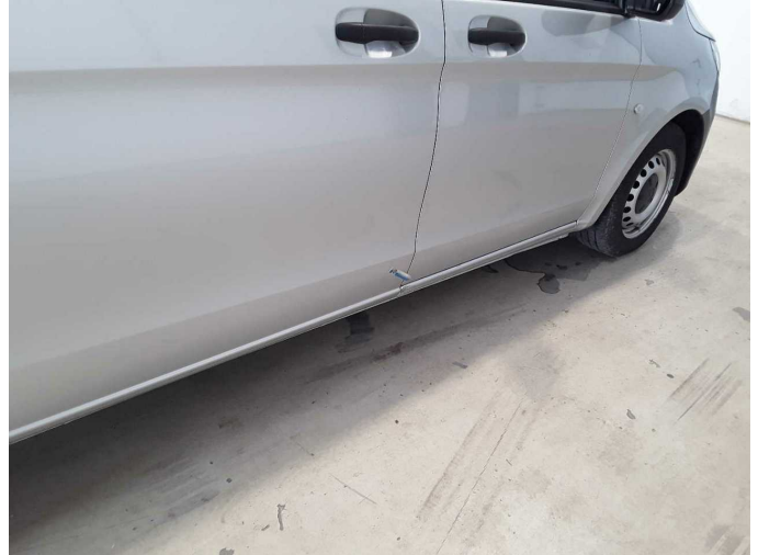
Damage 15: Sill - right side: Sill - Dent / paintcoat damage - Repair and paint
