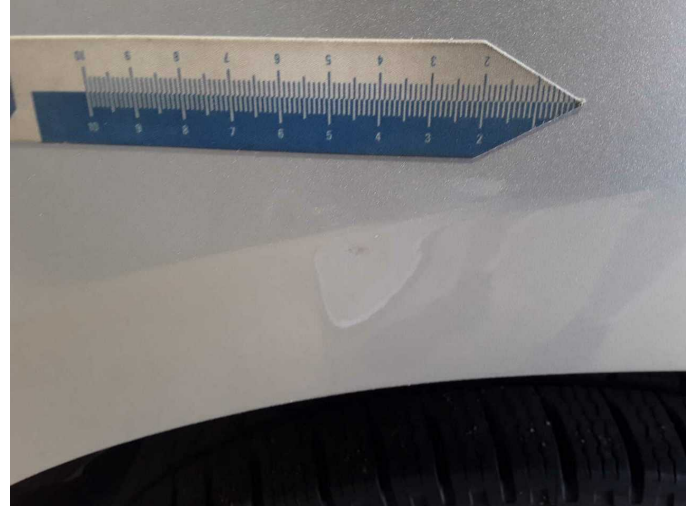
Damage 5: Side panel - rear left side: Side panel - Dent / paintcoat damage - Smart repair
