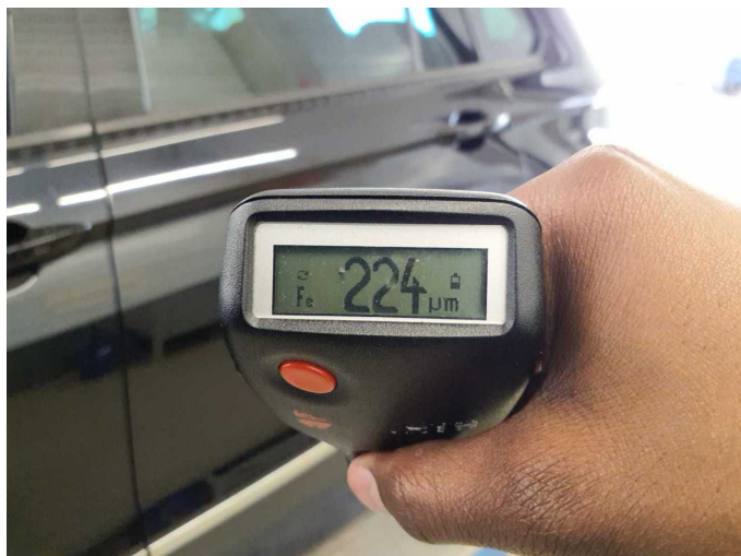
Repainting 1: Door - rear left side
