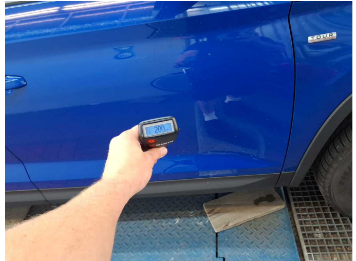
Repainting 1: Door - rear left side, Door - front left side, Door - front right side
