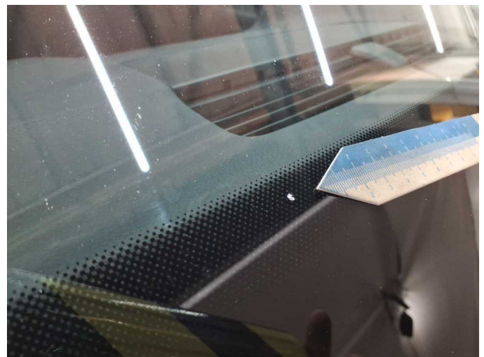
Damage 4: Vehicle glazing: Windscreen - Stone chips - Replace
