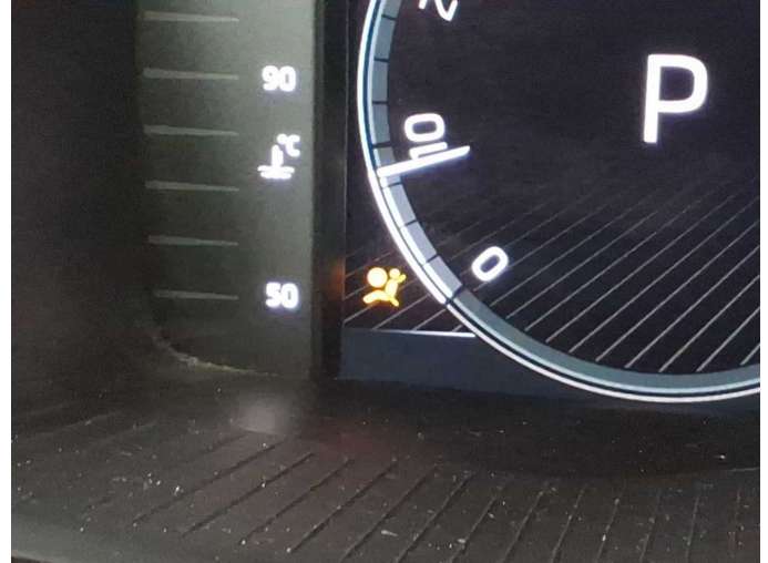
Damage 2: Instrument panel: Indicator light (Airbag) - on - Perform
