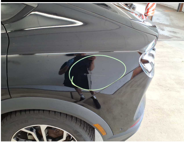
Damage #9: Side panel - rear left side: Side panel - Dent / paintcoat damage - Repair and paint
