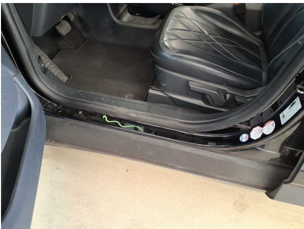
Damage #5: Door - front left side: Door seal - Damaged - Replace
