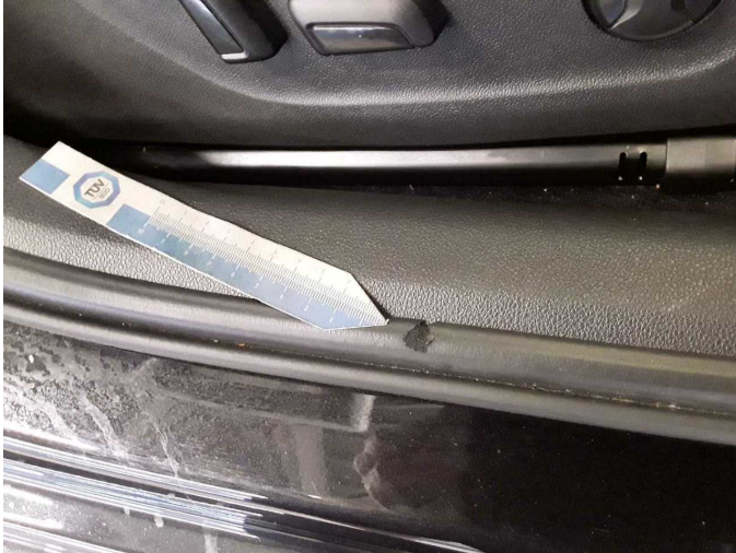
Damage 4: Cab: Door rubber seal - right side - Damaged - Replace
