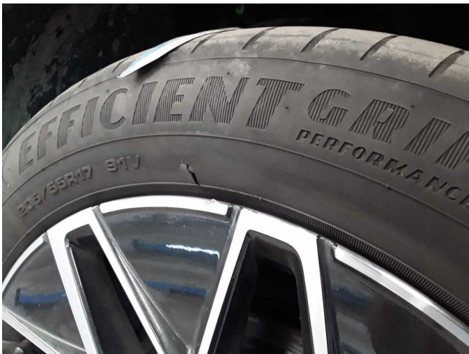
Damage 2: Wheel / tyres: Tyre - front right side - Porous / cracked - Replace
