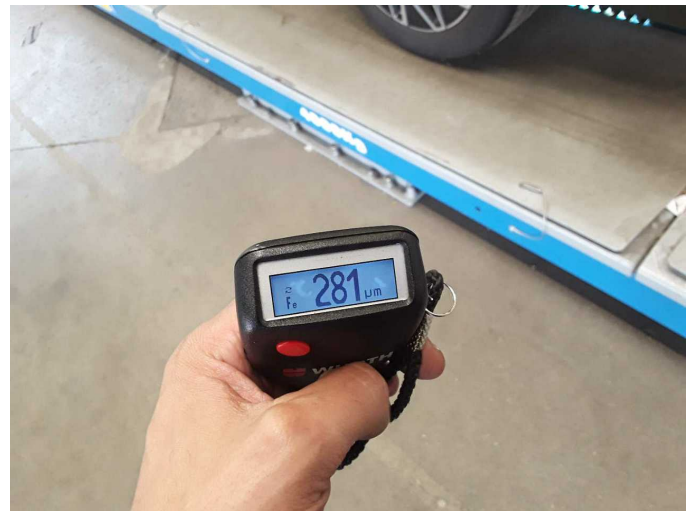
Repainting 1: Boot lid / rear door, Side panel - rear left side, Door - front right side
