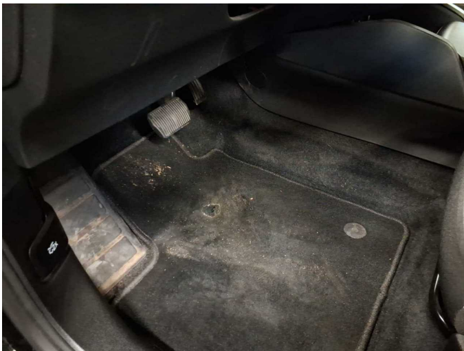
Damage 3: Trim / covers: Floor mats - Holes - Replace
