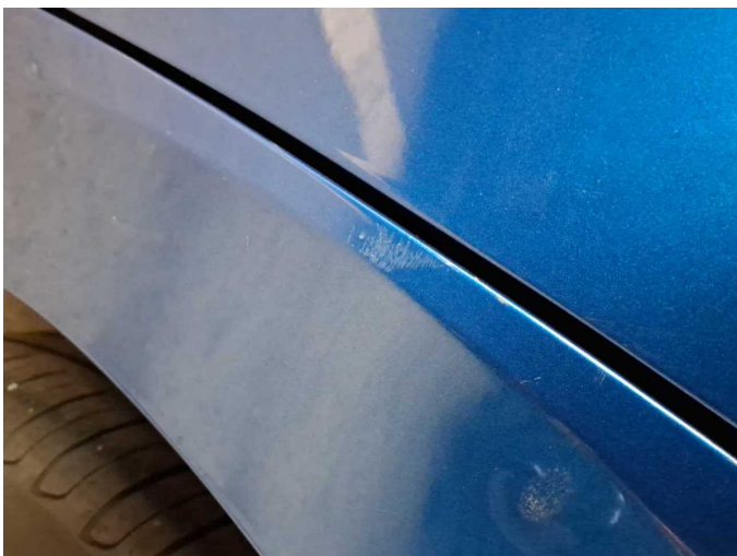
Damage 2: Side panel - rear left side: Side panel - Dent / paintcoat damage - Repair and paint
