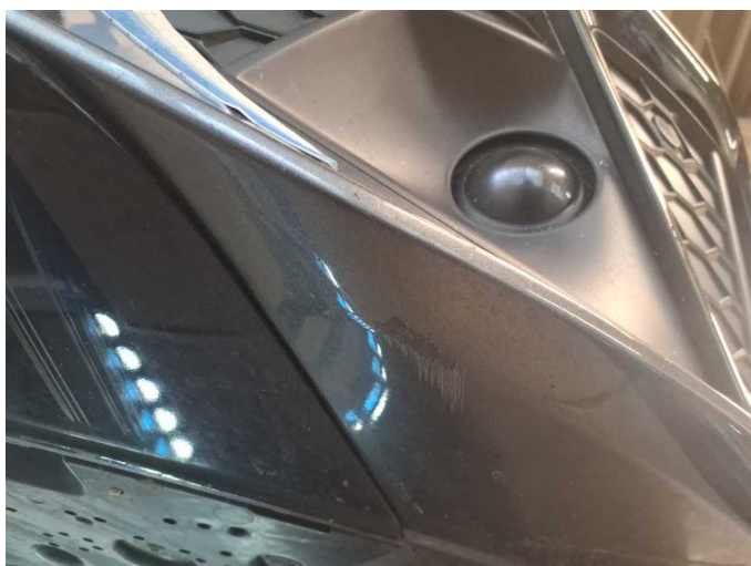
Damage 8: Front bumper: Front bumper - Scratched - Paint
