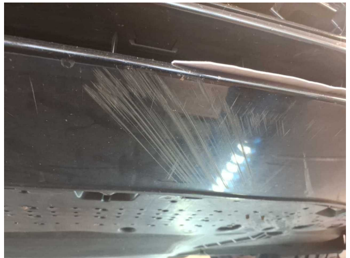
Damage 8: Front bumper: Front bumper - Scratched - Paint
