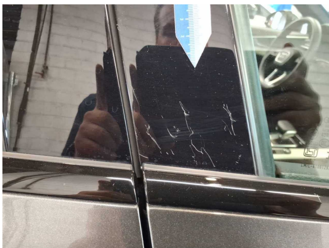
Damage 3: Door - front right side: Brightware - upper - Scratched - Smart repair
