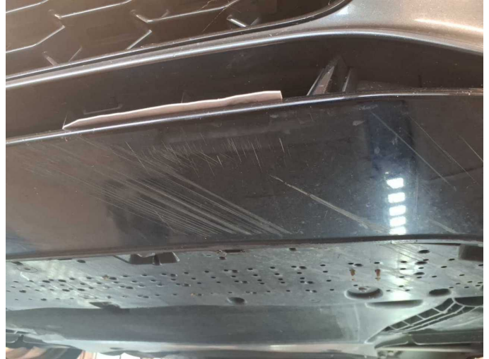
Damage 8: Front bumper: Front bumper - Scratched - Paint
