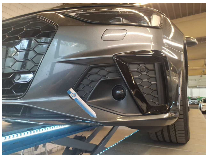
Damage 8: Front bumper: Front bumper - Scratched - Paint
