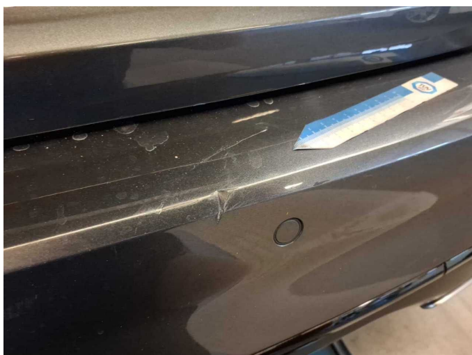
Damage 12: Rear bumper: Rear bumper (Fhgz. mit Sideassist) - Scratched - Replace
