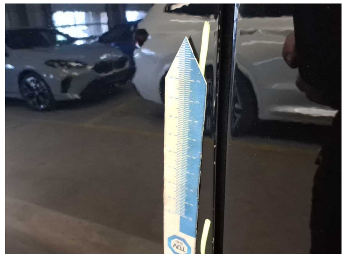
Damage 11: Door - front left side: Door - Dent / paintcoat damage - Repair and paint
