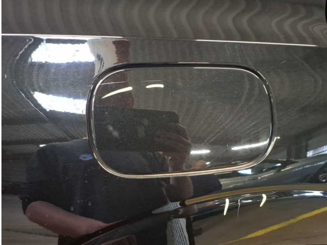
Damage 4: Fuel system: Tank cap - Scratch(es) - Smart repair
