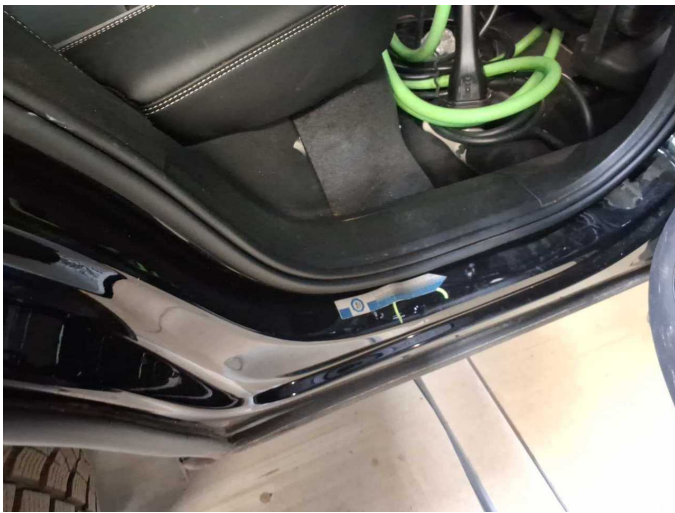
Damage 2: Side panel - rear right side: Sill - dent(s) - Smooth repair work
