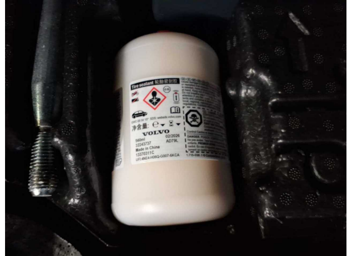
Damage 1: Equipment: Tirefit filler - Expired - Replace
