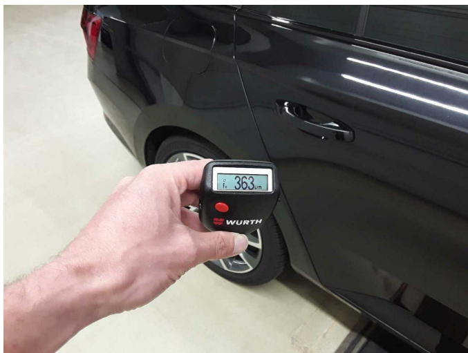
Side panel - rear right side: 363 µm
