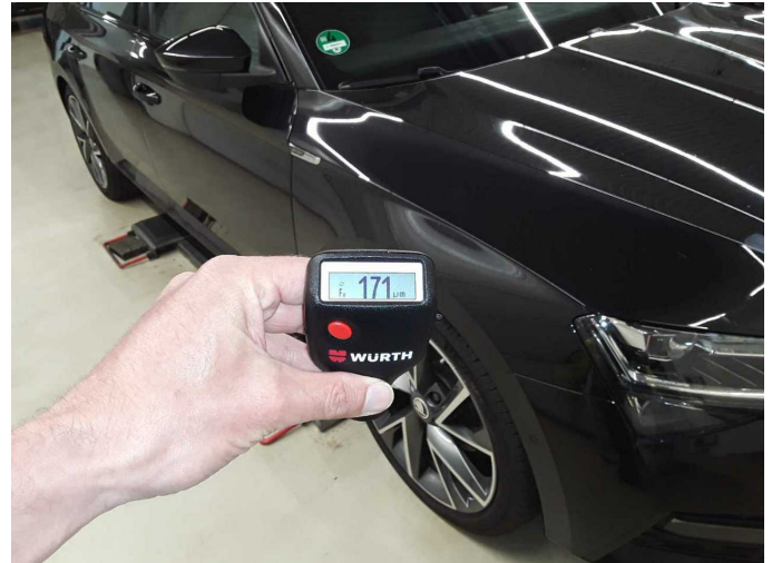
Mudguard - right side: 171 µm
