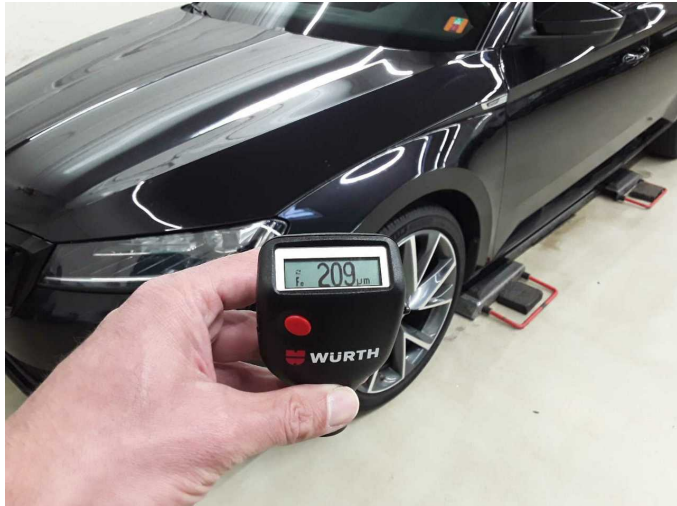
Mudguard - left side: 209 µm
