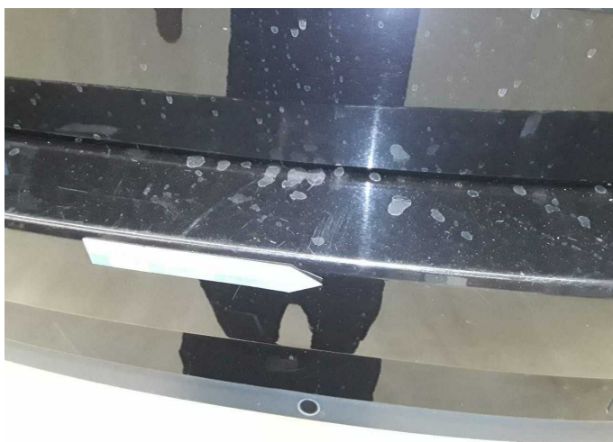
Damage 5: Rear bumper: Rear bumper - Scratched - Repair and paint
