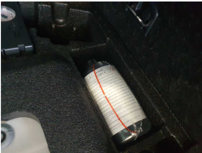
Damage 1: Equipment: Tirefit filler - Expired - Replace
