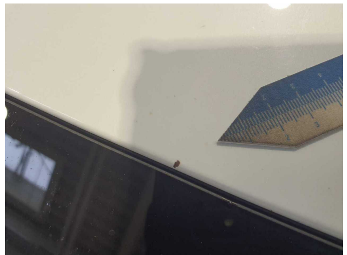
Damage 6: Roof: Roof - Stone chips - Smart repair
