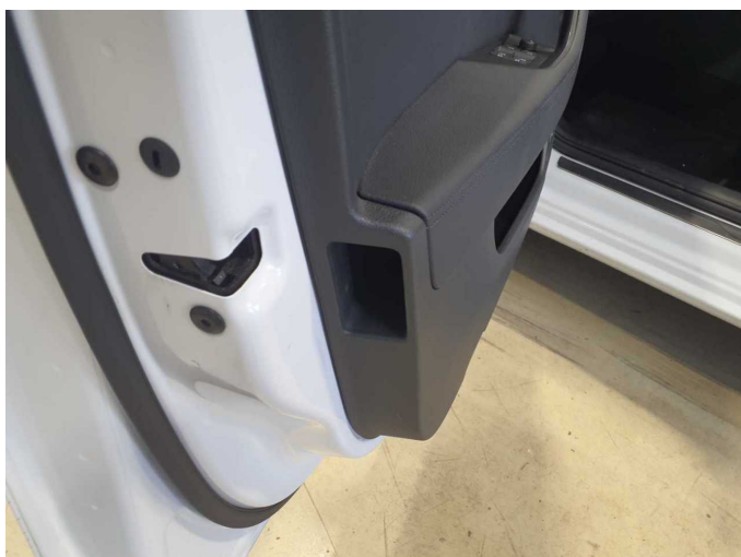
Missing part 1: Equipment: Umbrella - Missing - Replace
