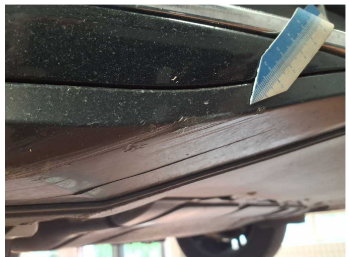
Damage 5: Front bumper: Front bumper (Blende rechts Erneuern / Blende Links A+E) - Scratched - Paint
