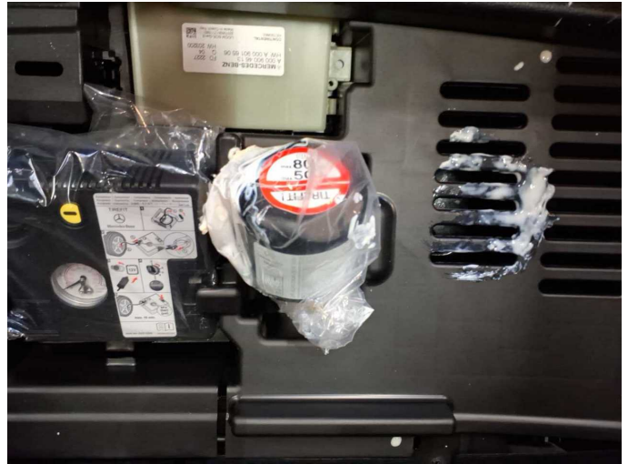
Damage 1: Equipment: Tirefit filler - Leaking - Replace
