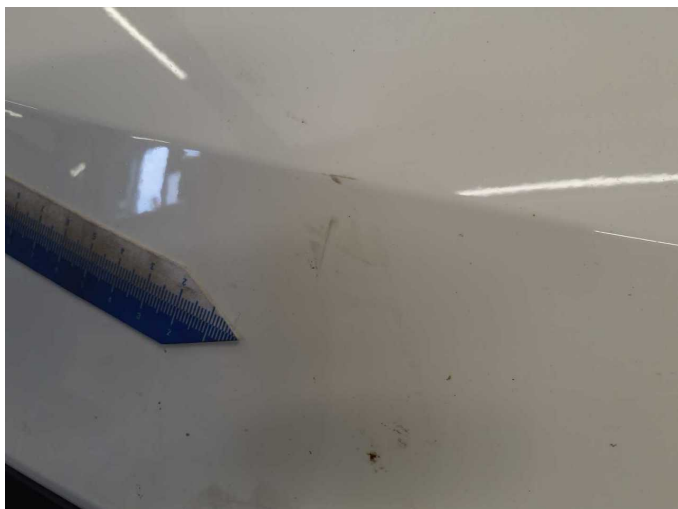
Damage 7: Front bumper: Front bumper - Scratch(es) - Paint
