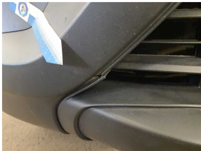
Damage 6: Front bumper: Front bumper - Broken / torn - Replace
