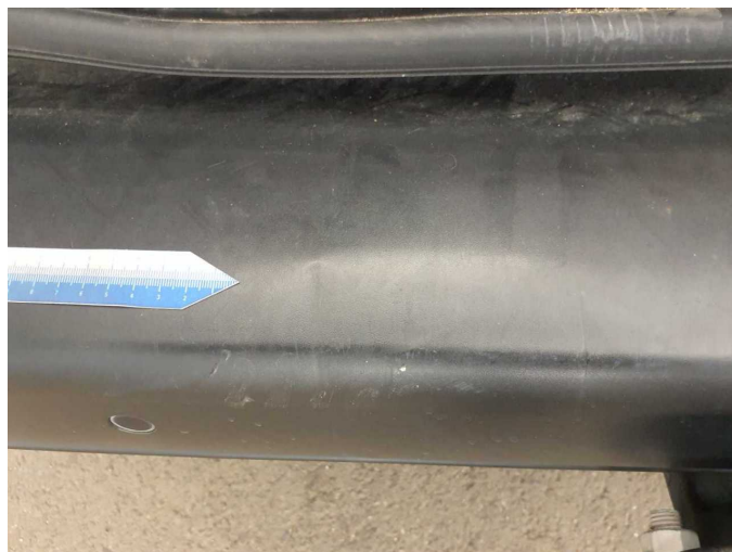
Damage 1: Rear bumper: Rear bumper - Deformed - Loss in value
