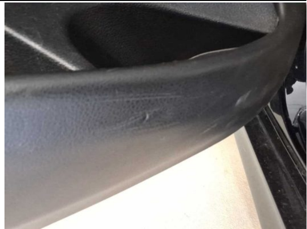
Damage #11: Trim / covers: Door trim - front left side - Damaged - Loss in value
