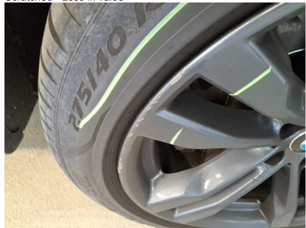
Damage #15: Wheel / tyres: Alloy rim - front right side - Scratched - Loss in value
