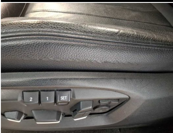
Damage #8: Seat - front: Seat cover - left side - Porous / cracked - Loss in value
