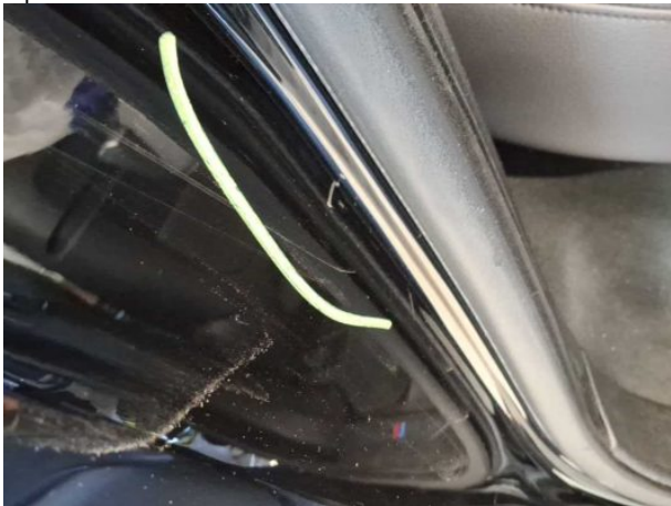
Damage #17: Side panel - rear right side: Sill - Scratched - Smart repair
