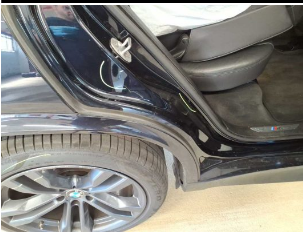
Damage #17: Side panel - rear right side: Sill - Scratched - Smart repair
