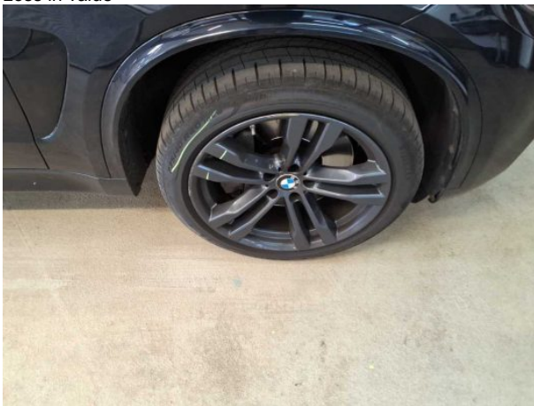
Damage #15: Wheel / tyres: Alloy rim - front right side - Scratched - Loss in value
