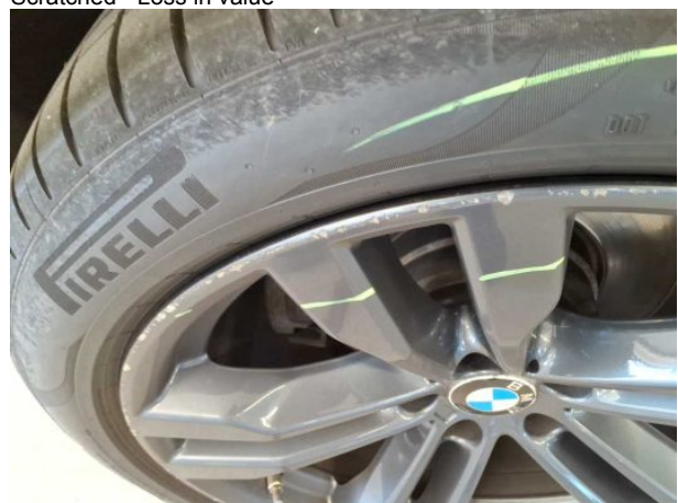
Damage #16: Wheel / tyres: Alloy rim - rear right side - Scratched - Loss in value
