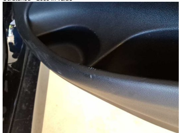
Damage #10: Trim / covers: Door trim - rear right side - Scratched - Loss in value
