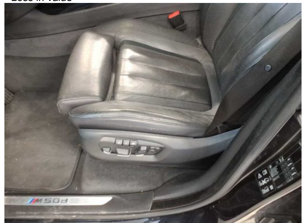
Damage #8: Seat - front: Seat cover - left side - Porous / cracked - Loss in value
