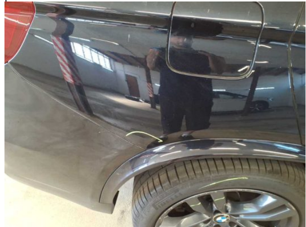
Damage #3: Side panel - rear right side: Side panel - Scratch... - Cover / polish
