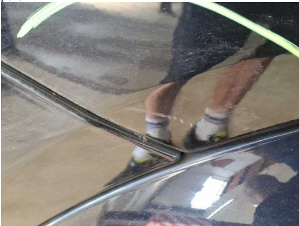
Damage #3: Side panel - rear right side: Side panel - Scratched - Cover / polish
