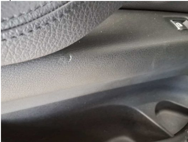
Damage #7: Trim / covers: Door trim - rear left side - Damaged - Loss in value
