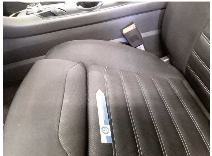
Damage 3: Seat - front: Seat cover - left side - Worn - Smart repair
