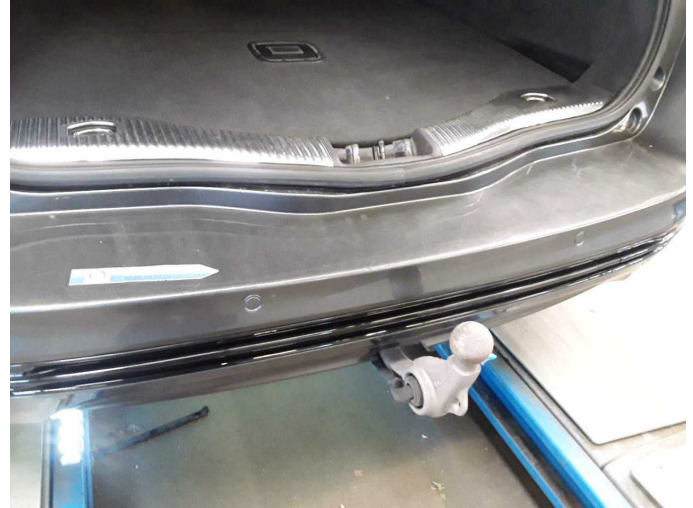
Damage 7: Rear bumper: Rear bumper - Scratch(es) - Paint
