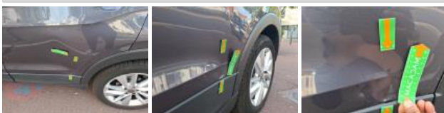
Door RL, Dent(s), Repair and paint (complete)
