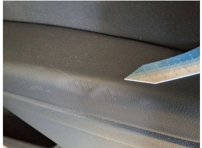
Damage 4: Trim / covers: Door trim - rear right side - Deformed - Replace
