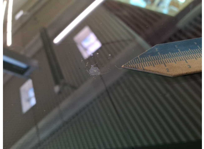
Damage 6: Vehicle glazing: Windscreen with lane departure assistant (Steinschlag + Kratzer) - Unprofessionally repaired - Replace
