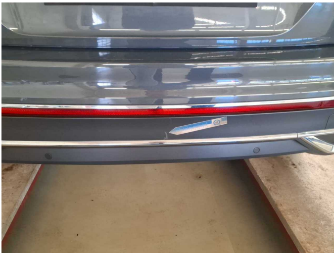
Damage 2: Trim / covers: Trim / covers (Stossfänger hinten unten) - Scratch(es) - Smart repair
