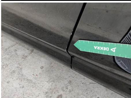
Tür / Vorne Links / Kratzer
