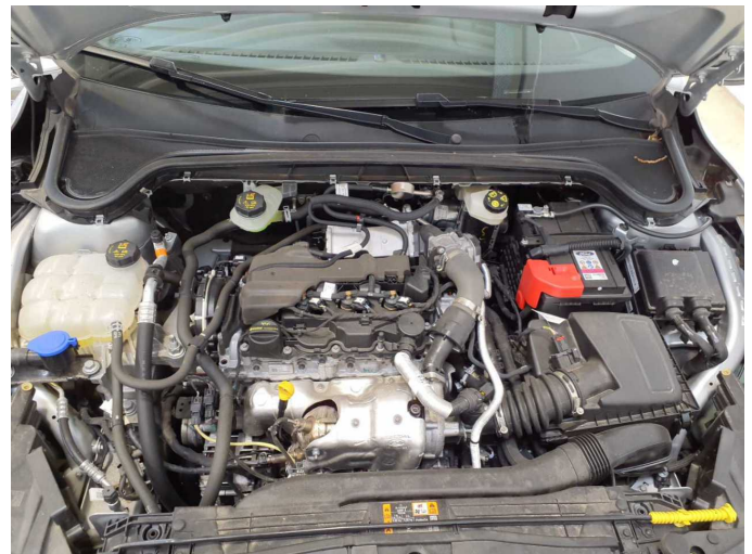
Missing part 2: Engine: Engine cover - Missing - Replace
