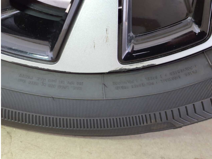
Damage 3: Wheel / tyres: Wheel cover - front left side - Scratch(es) - Replace
