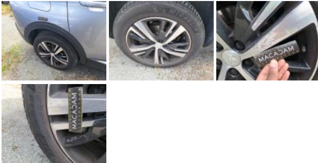
Tyre RR, Out of tolerance, Replace
