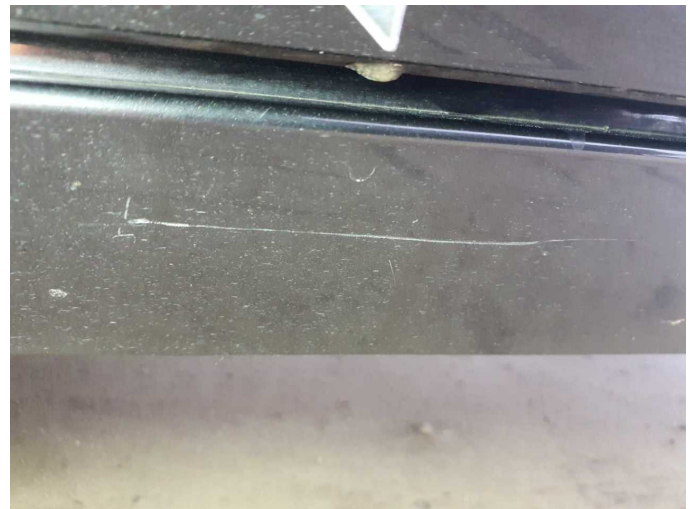
Damage 4: Sill - left side: Trim - Scratch(es) - Smart repair
