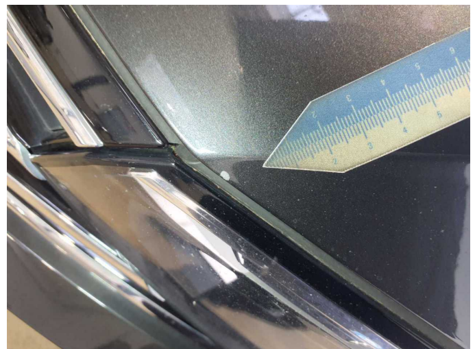
Damage 5: Bonnet: Bonnet - Stone chips - Smart repair
