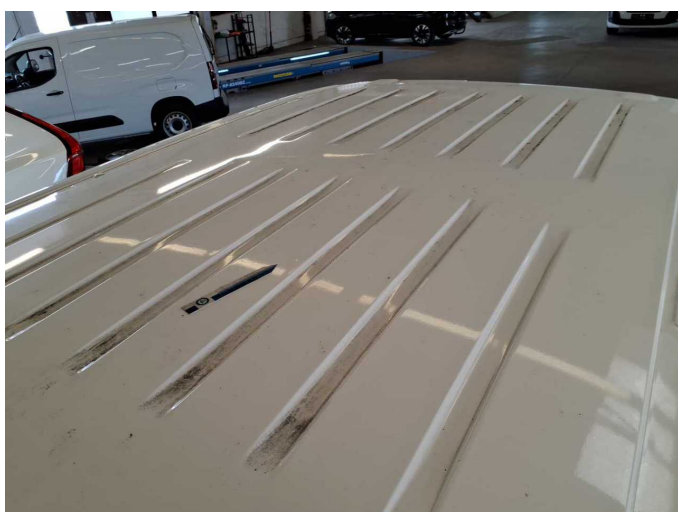
Damage 4: Roof: Roof - dent(s) - Smooth repair work
