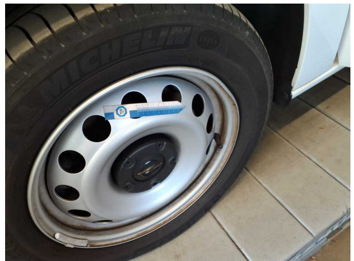
Damage 2: Wheel / tyres: Wheel rim - front left side - Deformed - Replace
