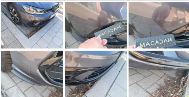
Bumper moulding F, Scratch(es), Repair and paint (complete)
