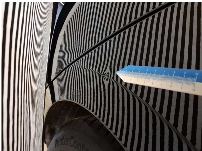
Damage 20: Side panel - rear left side: Side panel - Dent / paintcoat damage - Repair and paint
