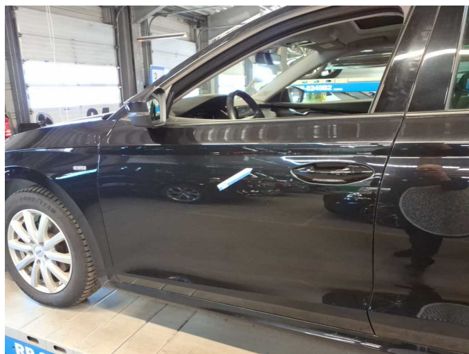
Damage 19: Door - front left side: Door - Dent / paintcoat damage - Repair and paint
