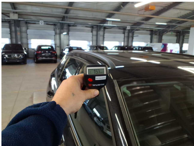
Repainting 1: Roof rail - right side
