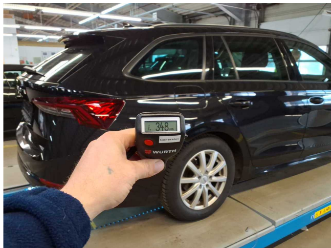
Repainting 2: Side panel - rear right side
