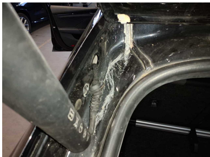
Damage 6: Body: D-pillar - left side - Scratched - Smart repair
