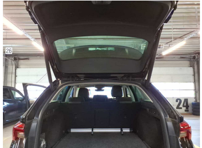
Damage 17: Boot lid / rear door: Gas pressure damper (Motor, links + Halterinkl. inkl. Halter) - Loose - Replace
