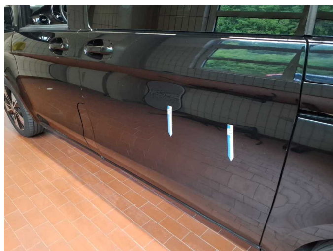
Damage 9: Sliding door - left side: Sliding door with glass panel - Scratch(es) - Paint
