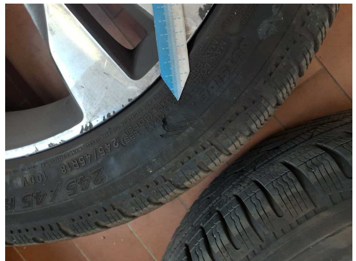
Wear and tear 5: 2nd wheel set: 1 tyre - Broken / torn - No deduction
