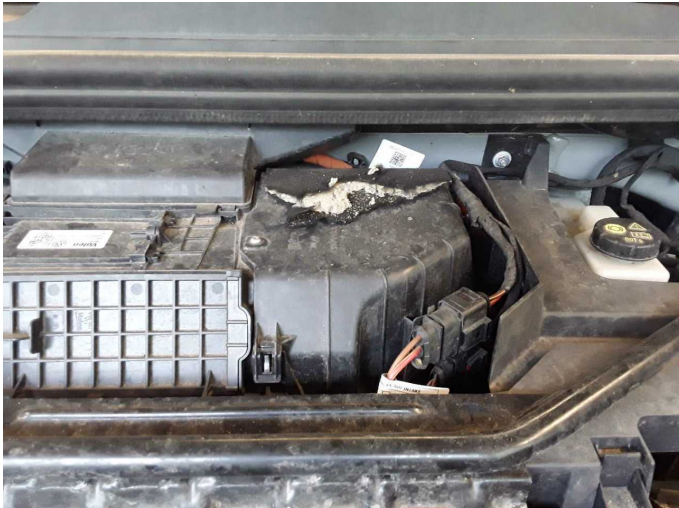
Damage 1: Engine: Engine cover - Damaged - Replace
